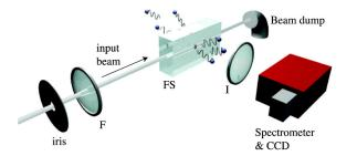
FIG. 1 (color online). Experimental layout used for detecting analogue Hawking radiation. The input laser pulse is focused into a sample of fused silica (FS) using an axicon or lens (F). An imaging lens (I) collects the photons emitted at 90° and sends them to an imaging spectrometer coupled to a cooled CCD camera.
