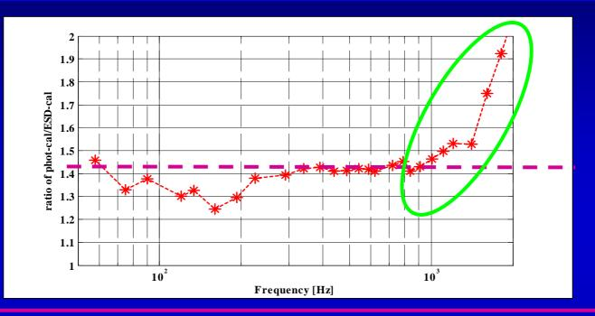
1. Absolute deviation of 40 % (amp in DER\_DATA\_H is smaller than expected) *Candidate: PPD and IFO not hitting center of testmass.*
