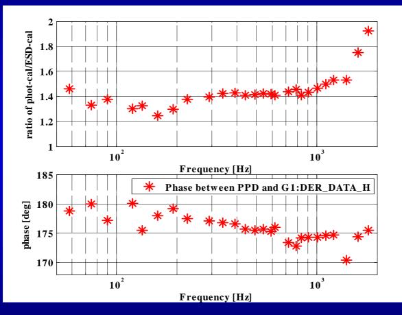
Due to the pendulum response the mirror is 180° out of phase with the applied light modulation (quite unintuitive).
