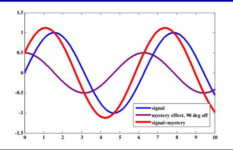
The resulting amplitude gets larger. In contrast we observe in the experiments a smaller amplitude than expected.
