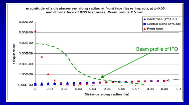
• The displacement needs to be weighted by the overlap of the main IFO beam. For now I will use 1e-9 m/2.77N.
