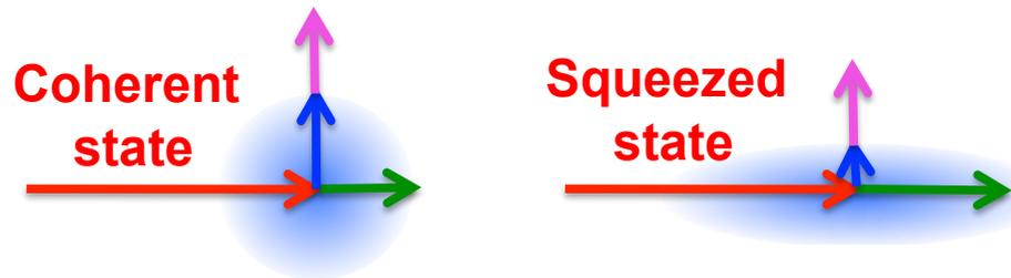
Injection of squeezed light will reduce photon shot noise / quantum noise.
