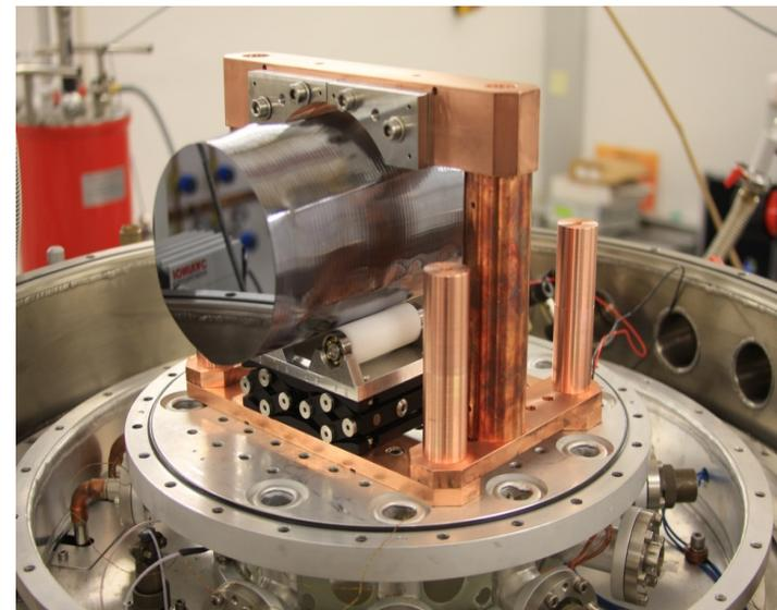
There is not only thermal noise from the test mass substrates, but also from the mirror coatings (amorphous dielectric materials). This noise scales again with temperature and loss, but also with the number of the layers.
