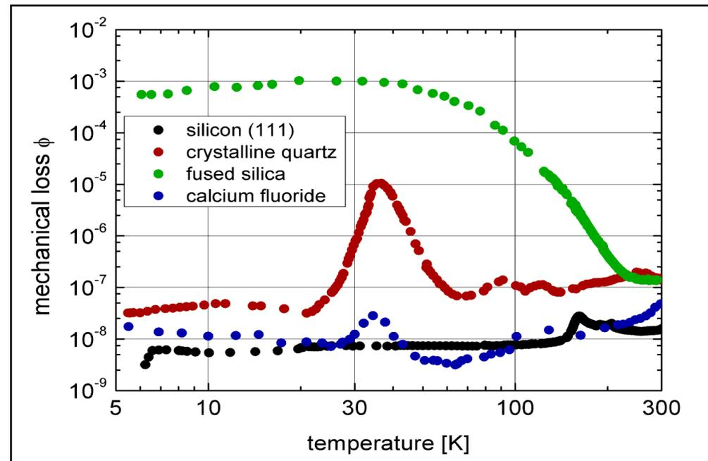
Fused silica – as the material currently in use – is not suited for cryogenic operation due to its large loss peak.
