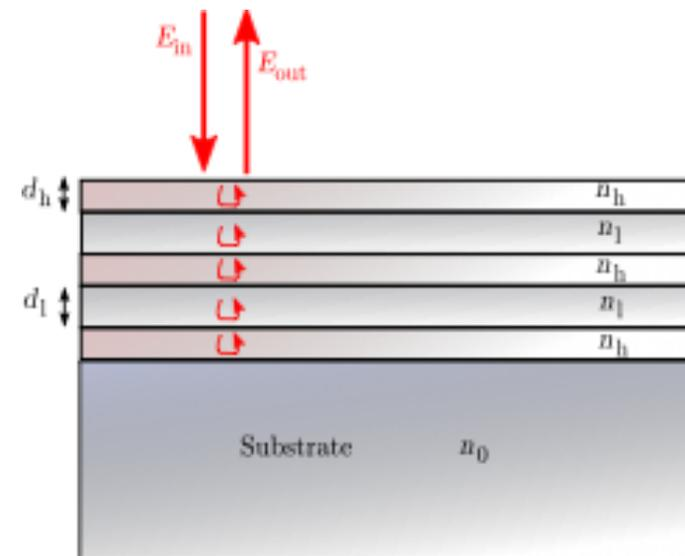
**Idea: replacing the dielectric (lossy) multilayer stack by a monocrystalline silicon micro structure**
