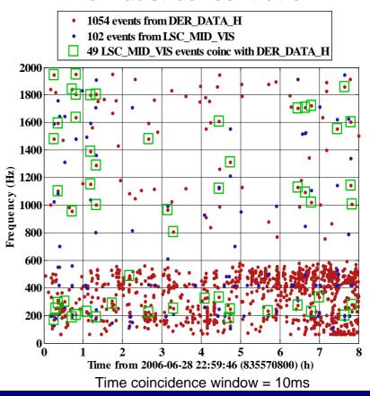
When dust is falling through the main output beam, coincidence glitches are induced to H and  $P_{DC}$ .
