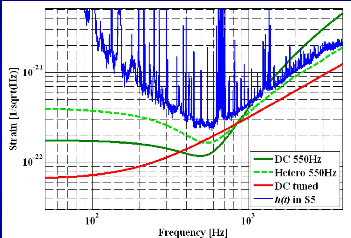
Tuned DC-readout might be a useful precursor for GEO-HF (option for squeezed light input => no filter cavity necessary)
