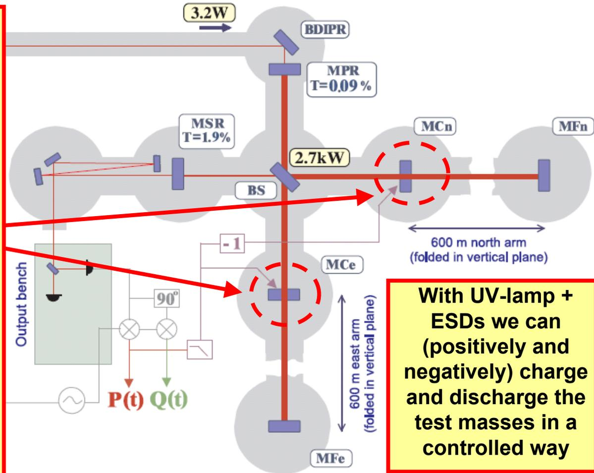
With UV-lamp + ESDs we can (positively and negatively) charge and discharge the test masses in a controlled way
