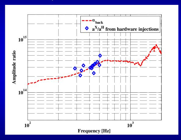
Around 1.8 kHz MID\_VIS is especially sensitive to GW-like signals.
