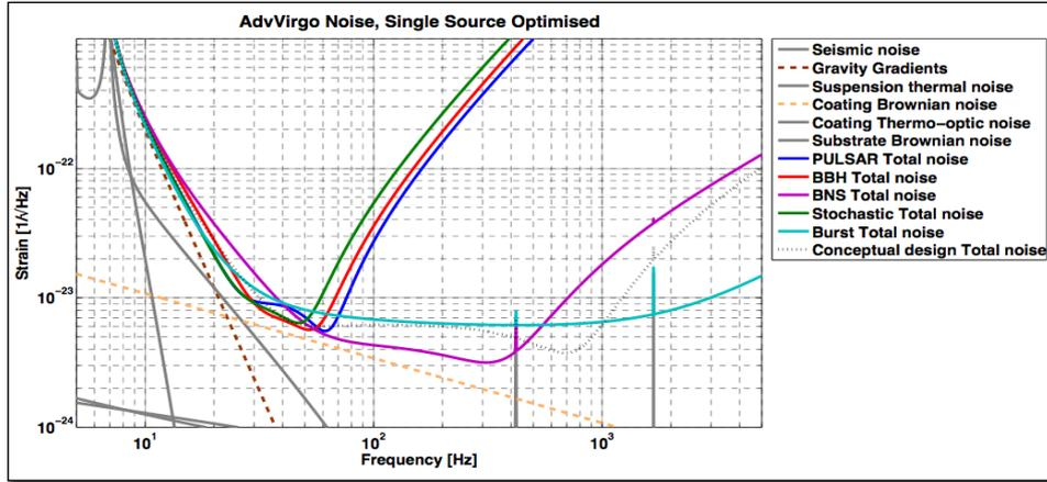
Curves show the optimal sensitivity for a single source type.
