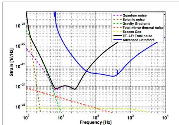
As mirror TN is no longer limiting, one can relax the assumptions on the material parameters and the beam size...
