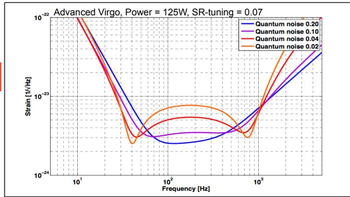
Resonances are less developed for larger SR transmittance.
