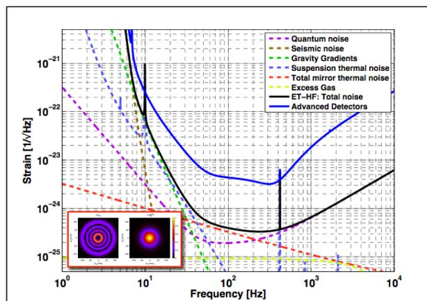
Coating Brownian reduction factors (compared to 2G): 3.3 (arm length), 2 (beam size) and 1.6 (LG33) = 10.5
