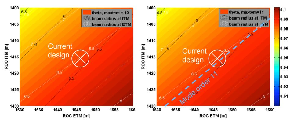
The higher order mode closest to being resonant in the arm cavities is of the order 11.
