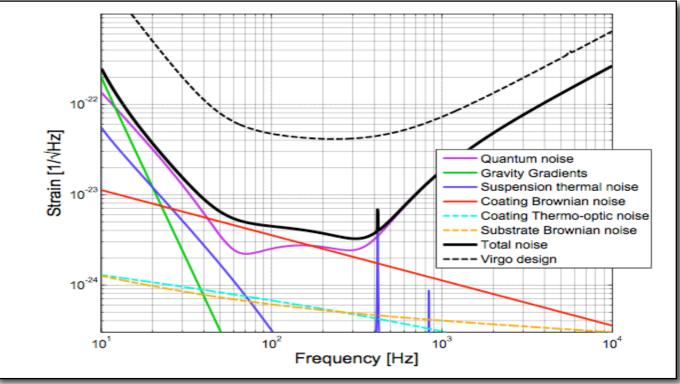
Coating Brownian noise is the limiting noise source in the mid frequency range.
