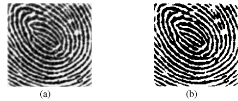
Fig. 7. Comparison of fingerprint images before and after using Otsu. (a) Original fingerprint image. (b) Fingerprint image using Otsu.
