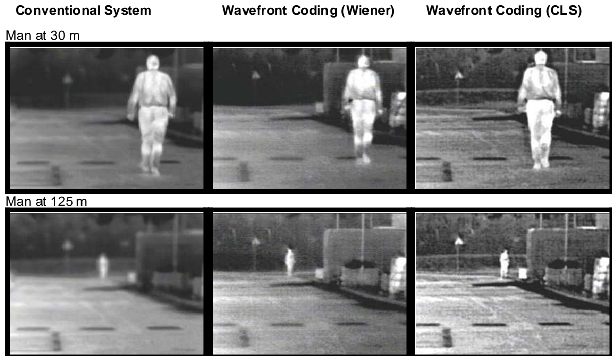
Figure 1. Captured images comparing similar scenes for conventional system focused at 20 m, wavefront coding system using Wiener algorithm and wavefront coding system using CLS algorithm
