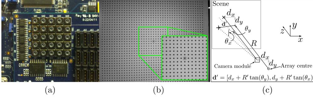
Fig. 1. (a) The low-cost miniature camera array. (b) Image of the calibration chart. Close observation shows that there is a degree of visible distortion in the system. (c) Geometry for inferring camera module rotation about  $x$  and  $y$ .
