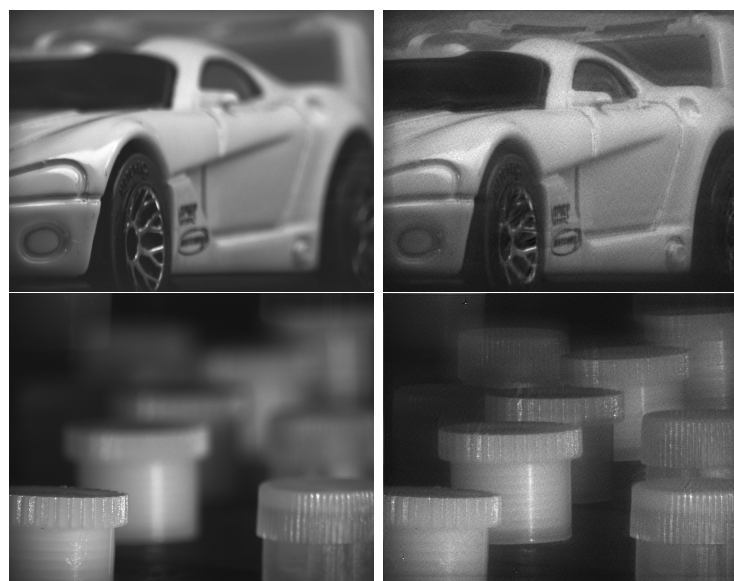
Figure 9. Images of deep scenes. Left images are non-coded and right images are obtained with codification (using cubic phase mask of \alpha = 5 ) and restoration (using the parametric Wiener filter with k = 0.005 ).
